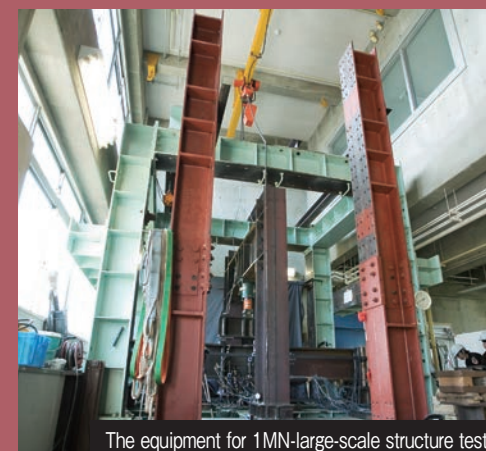
Bending and shearing examination of the reinforced concrete beam
