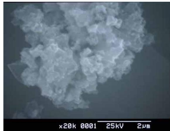
Fig.23. SEM images of the resulting  $\text{LiFePO}_4/\text{C}$  powders.
